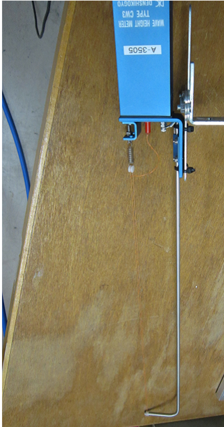
Fig. 2.4: Photograph of reference sensor
