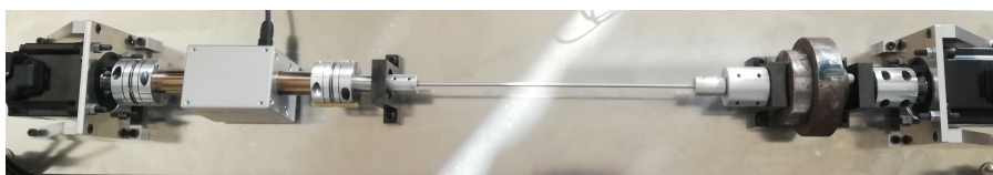
Fig. 2.7: Experiment system using torque sensor(top view)
